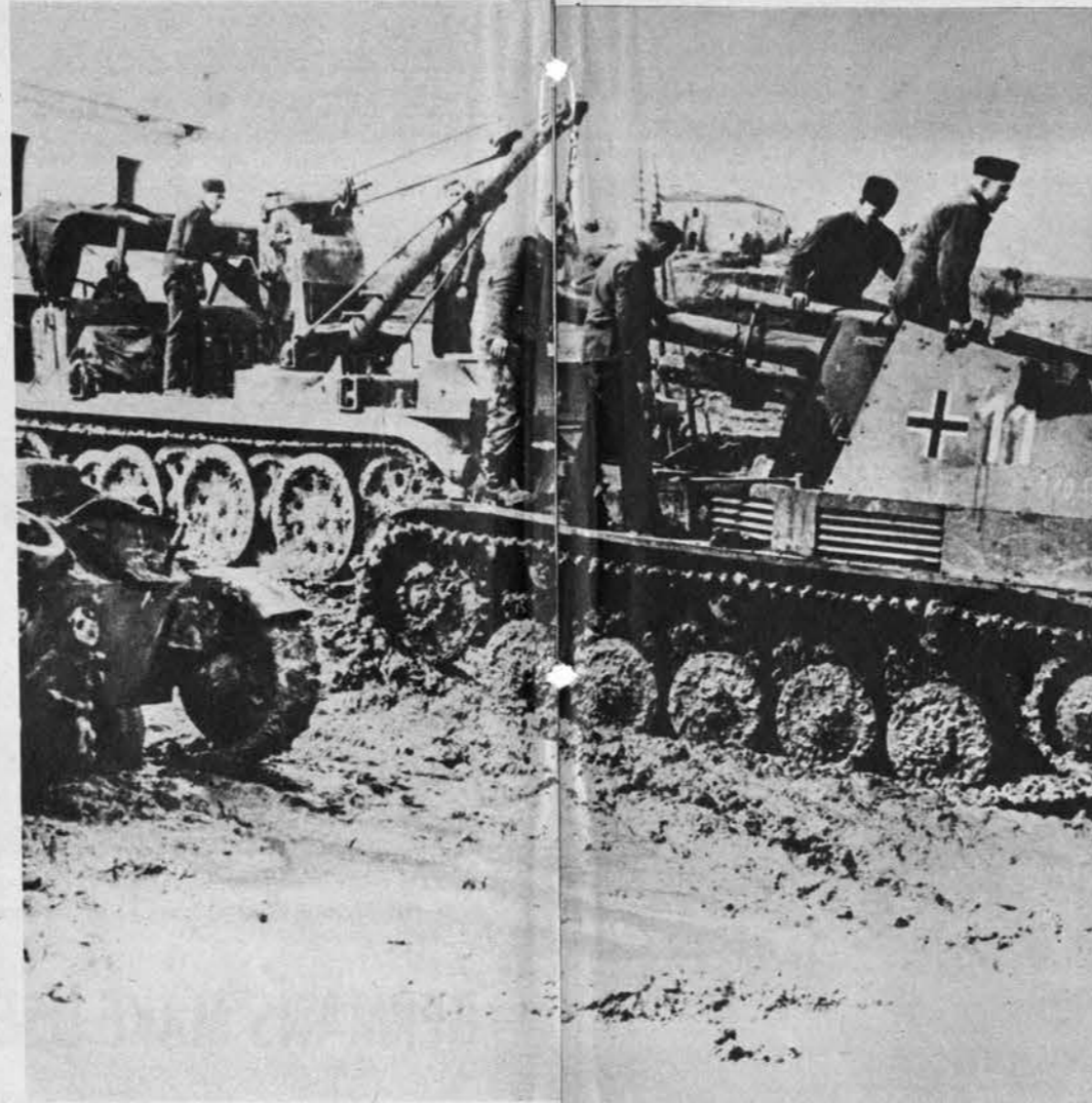
German tank repair unit recovers a bogged-down Wasp from mud. Buffer and recuperator of the 105-mm. howitzer project well beyond
